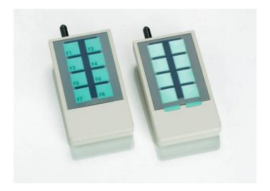
The 8-button transmitter FRT-HS 8 is a handheld unit for RF transmission of up to 8 commands, which can be received and indicated visually and/or by tone or which can switch up to 8 relays. The 8 buttons can either be imprinted with "F1" ... "F8" or can be blank, having two detachable strips for an individual inscription.
