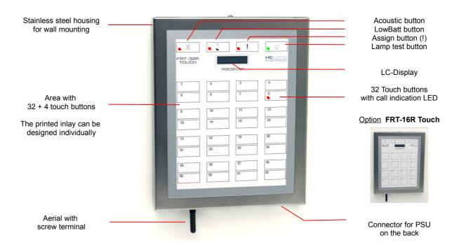
The FRT-32R-Touch is a wireless Call Indication Panel for up to 32 call buttons (table transmitters et al.). The slim and easy to clean stainless steel housing can be fixed to the wall by 2 screws like a picture. Incoming calls from up to 32 call buttons are indicated at the respectively assigned buttons and the LCD is showing all calls in order of its reception.
